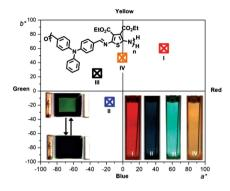
Thermal polymerization of a conjugated polymer is performed directly on the device electrode using solution-processable monomers. The resulting immobilized polymer is electroactive and it is reversibly switched electrotrochemically between its colored states. The polymer is successfully used as the electrochromic layer in a working device with repeated color switching.
