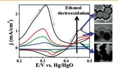
Hierarchical MgFe-layered double hydroxide (LDH) microspheres with tunable interior structure (hollow, yolk–shell, and solid) are synthesized by a facile and cost-effective surfactant-templated method. The resulting hollow LDH microspheres yields largely enhanced activity as well as robust durability towards ethanol electro-oxidation, owing to the significantly improved mass transport and faradaic redox reaction.
