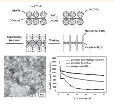
A graphene-based mesoporous SnO<sub>2</sub> composite is prepared via in situ growth of mesoporous SnO<sub>2</sub> on the graphene surface using cetyltrimethylammonium bromide (CTAB) as a template. Because of the high specific surface area and stable mesostructure of SnO<sub>2</sub> nanocrystalline on graphene, it displays higher reversible capacity, better cycle performance, and better rate capability compared to mesoporous SnO<sub>2</sub> and graphene-based non-porous SnO<sub>2</sub>.
