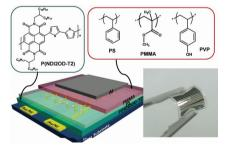
Highly stable top-gated organic nanofloating-gate memory (NFGM) devices with quasi-permanent retention characteristics are fabricated using an n-type conjugated polymer. The best polymer NFGM devices show excellent memoryrelated characteristics along with a wide memory window, a high on-off current ratio, and a long retention time.
