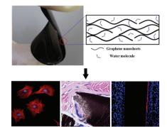
A self-supporting graphene hydrogel film prepared by a simple vacuum filtration technology is used as a unique experimental platform to study how graphene interacts with biological tissues both in vitro and in vivo. This graphene-based bulk material appears to be highly biocompatible, biodegradable, and osteoinductive, demonstrating graphene's potential for bone regenerative medicine.
